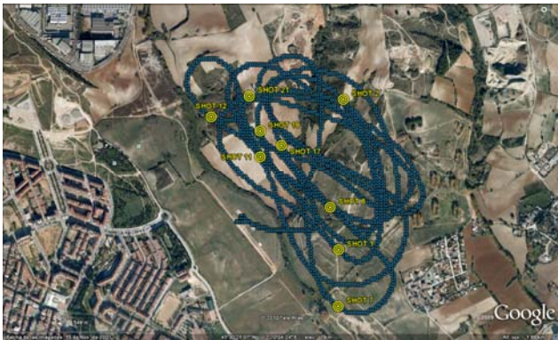
Figure 4. aircraft trajectory (blue dots) and the SiGe-based reflectometer successfully shots (yellow dots)
