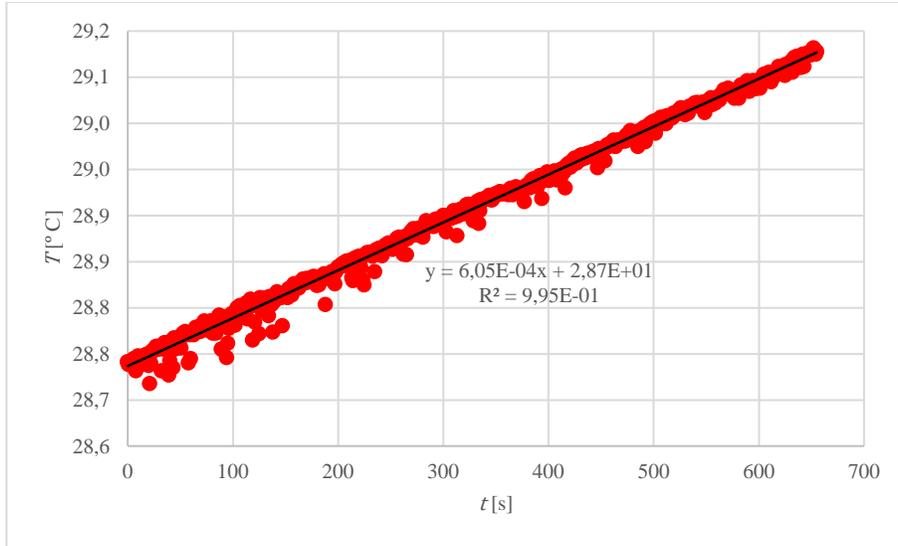
Figure 1. Water temperature inside the suction tank as a function of elapsed time with cavitation in the Venturi section, lineal trend line and equation.
