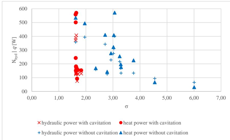
Figure .3 Hydraulic power with cavitation (crosses) and without cavitation (pluses), and heat power with cavitation (circles) and without cavitation (triangles) plotted as a function of the cavitation number. Red colour indicates cavitation while blue colour indicates no cavitation
