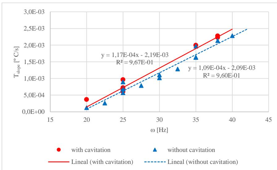
Figure 2. Temperature increase rate as a function of pump rotation frequency. Red circles indicate presence of cavitation while blue triangles indicate no cavitation in the system.
