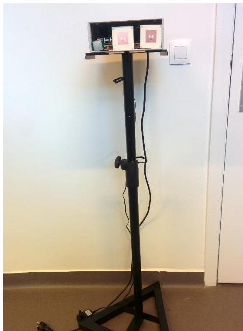
Figure 4.2.- Radar sensor placed in the stand near a wall.
