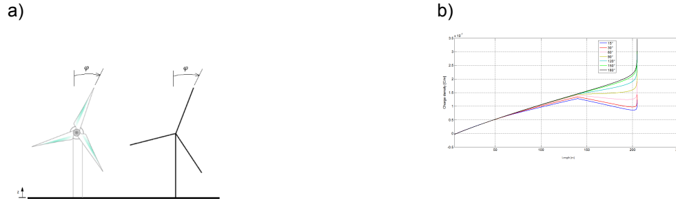
Figure 16. a) Simplified geometry of a wind turbine. b) Induced charge in a wind turbine under fair weather. (Adopted from [34]).
