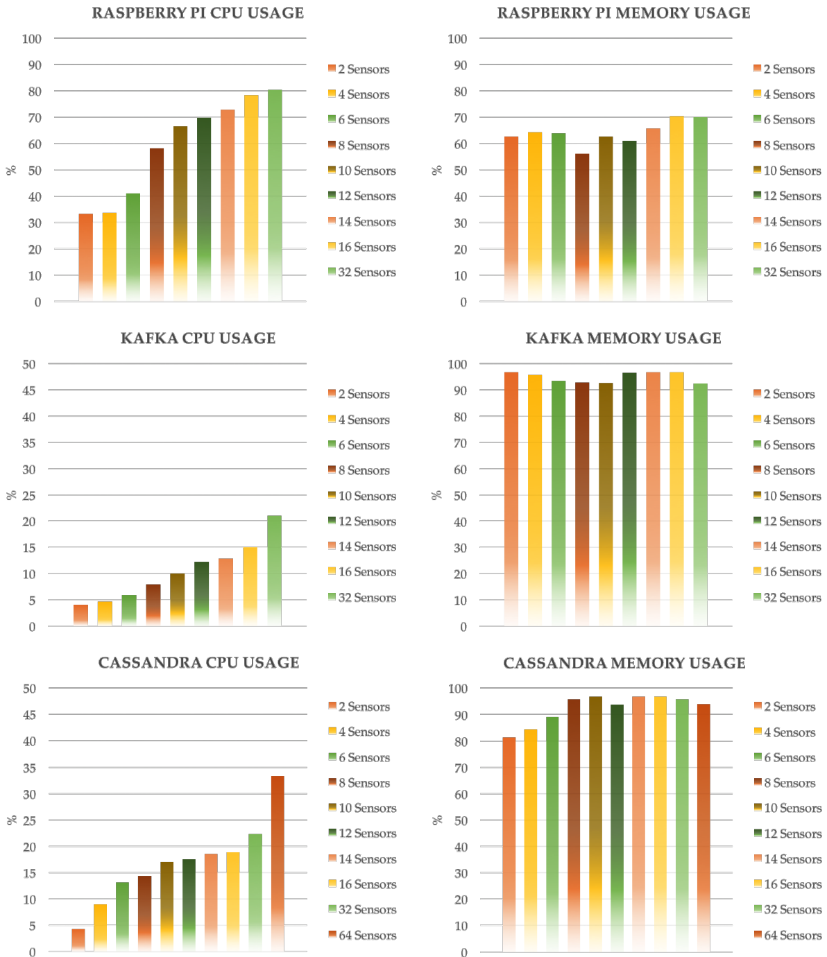
Figure 6.12: The bars represent the average values registered experimenting with an increasing number of sensors.
