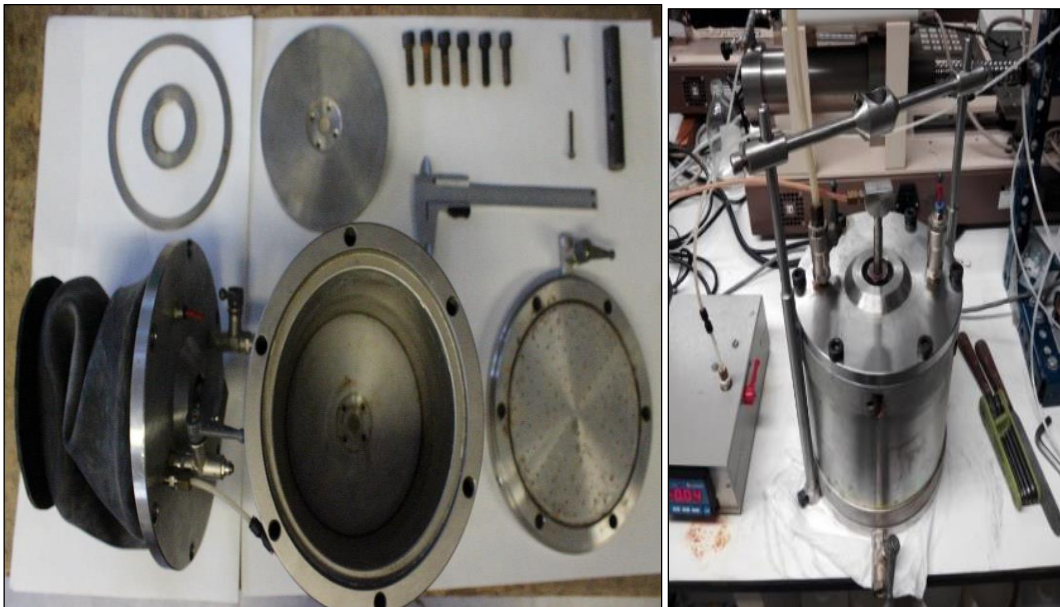
Figure 3-23: Oedometer cell provided at UPC Geotechnical Laboratory.
