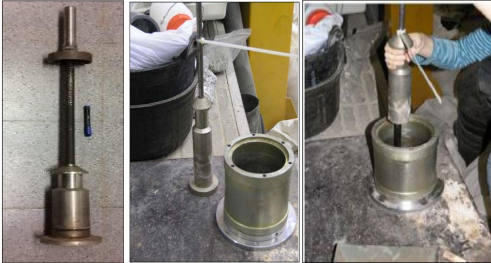
(a) Marshall compaction equipment.
