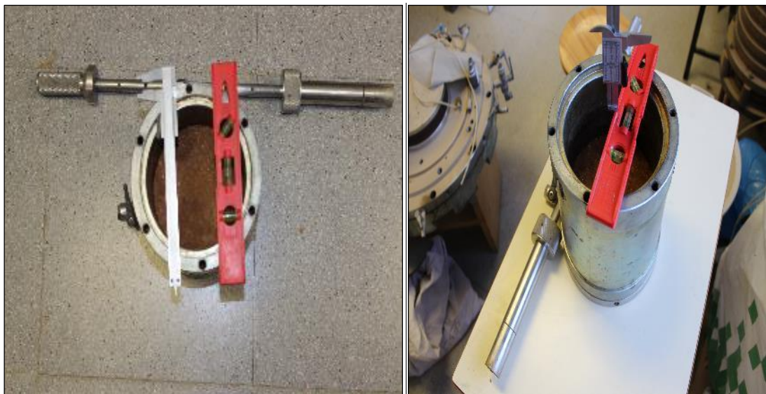
(b) Compaction equipment with Oedometric cell.
