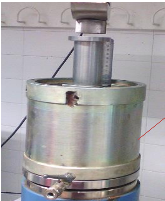
Figure 6-7: Provided cells and moulds to compact artificial fragments at UPC Geotechnical Laboratory.
