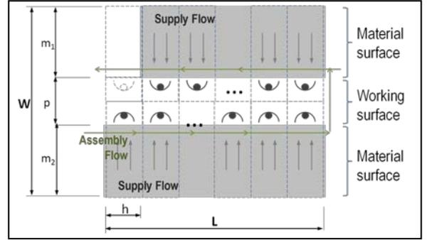
**Figure 2.** AGAIG topography for a number  $N$  of workstations.
