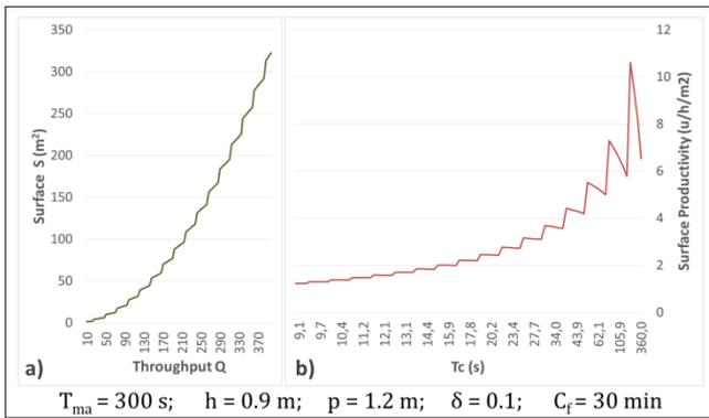
**Figure 3.** For typical industrial values: a) Surface ( $S$ ) vs. Throughput ( $Q$ ); b) Surface Productivity ( $SP$ ) vs. Cycle Time ( $T_c$ ).
