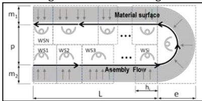
**Figure 1.** General topography for a U-SAL with  $N$  workstations.
