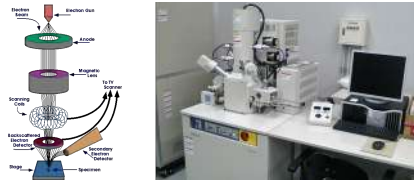
Figure 3.2: A - scheme of a standard SEM; B - Hitachi SU-8000 scanning electron microscope
