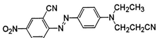
**Figure 1.** Structure of C.I. Disperse Red 73 (C.I. 11116, CAS 16889104, MW = 348.36 g·mol<sup>-1</sup>)
