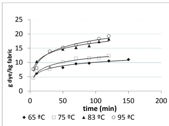
**Figure 7** Kinetics of dyeing with C.I. Disperse Blue 56 absorbed by polyester fabric at different temperatures in the presence of butyl acetate ( $16.666 \text{ g}\cdot\text{l}^{-1}$ ) and coumarin ( $0.666 \text{ g}\cdot\text{l}^{-1}$ ).
