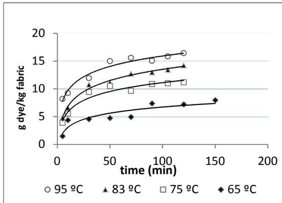
**Figure 5** Kinetics of dyeing with C.I. Disperse Red 73 absorbed by polyester fabric at different temperatures in the presence of butyl acetate ( $16.666 \text{ g}\cdot\text{l}^{-1}$ ) and coumarin ( $0.666 \text{ g}\cdot\text{l}^{-1}$ ).
