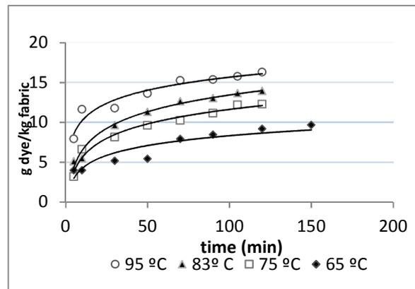
**Figure 6** Kinetics of dyeing with C.I. Disperse Red 73 absorbed by polyester fabric at different temperatures in the presence of butyl acetate ( $16.666 \text{ g}\cdot\text{l}^{-1}$ ) and *o*-vanillin ( $0.666 \text{ g}\cdot\text{l}^{-1}$ ).
