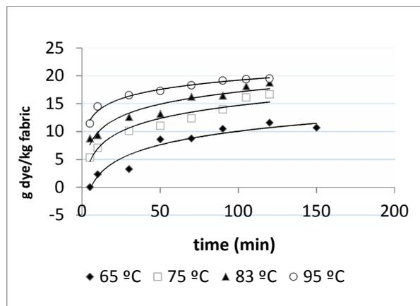
**Figure 8** Kinetics of dyeing with C.I. Disperse Blue 56 absorbed by polyester fabric at different temperatures in the presence of butyl acetate ( $16.666 \text{ g}\cdot\text{l}^{-1}$ ) and *o*-vanillin ( $0.666 \text{ g}\cdot\text{l}^{-1}$ ).
