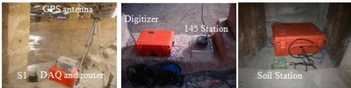
Figure 4. The dynamic system in operation: accelerometer S1, DAQ, router and GPS antenna (left); accelerometer 145-Station and digitizer (middle); and accelerometer Soil-station (right).
