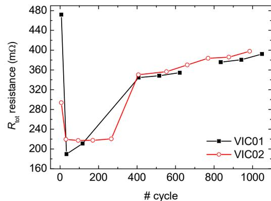
Fig. 2 - Total resistance evolution represented as the addition of polarization and diffusion resistances.
