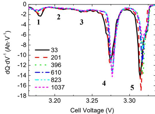
Fig. 3 - Incremental capacity analysis of a VIC cell (LFP) at different SoH at a C/25 discharge rate.
