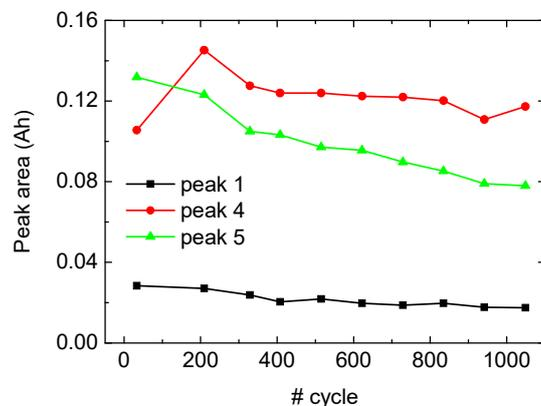
Fig. 4 - Evolution of the area of peaks obtained from ICA of a LFP cell at different SoH and at a C/25 discharge rate.
