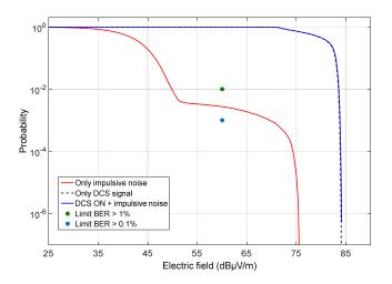
Fig. 2. APD standard measurement when the impulsive noise and the DCS signal are coexistnet, only the interference and only the DCS signal.
