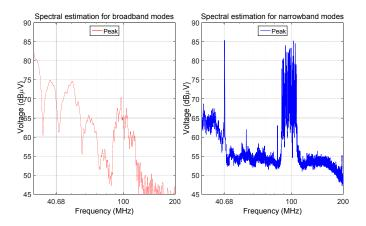
Fig. 5. Frequency domain results of the impulive noise and the narrow band DCS signals.
