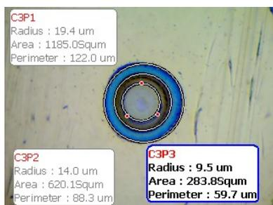
**Figure 6:** Typical laser spot produced with 355 nm UV laser.
