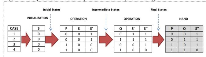
Fig. 5. Schematic sequence flow for NAND measurements involving two IMPLY operation steps.
