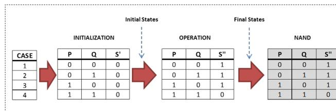
Fig. 9. Schematic flow sequence of one operation step procedure for NAND logic gate.
