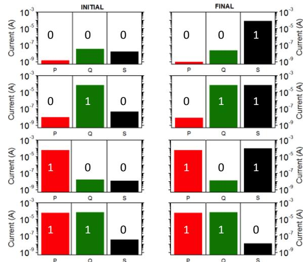
Fig. 8. NAND implementation with only one IMPLY operation step.
