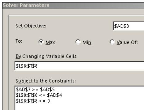
Figure 8: Non-linear solver parameters (objective and constraints)
