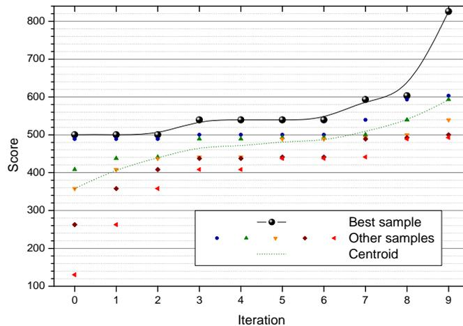
Figure 3: Evolution of samples score with Simplex iterations.
