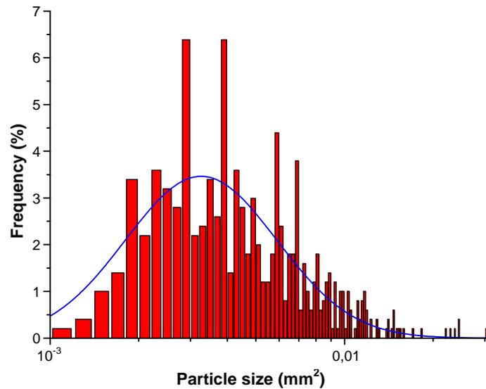
Figure 1: Size particle distribution of the sieved fraction expressed as surface of projected area.
