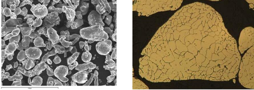
Figure 2: SEM image of the sieved powder morphology (left) and optical image of a particle's interior (right).
