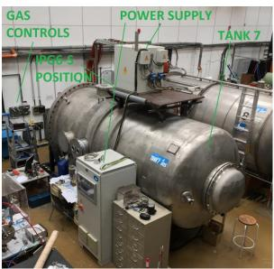
Fig. 3 IPG6-S refurbished facility
