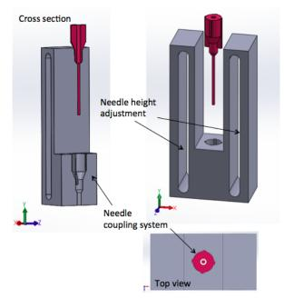
Figure  $2 \cdot 3d$  printed part to position the ink injector.
