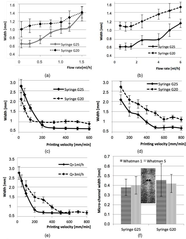
**Figure 5** Printing at constant velocity. (a) V=200 mm/min (b) 500 mm/min. (c) Printing at constant flow rate. 1ml/h (d) 3ml/h, in both cases G25 needle provides smaller line width (e) Printing with the G25 needle at different flow rates. According to the results, the optimum parameters are 800 mm/min and 1 ml/h (f) Minimum channel width vs. needle
