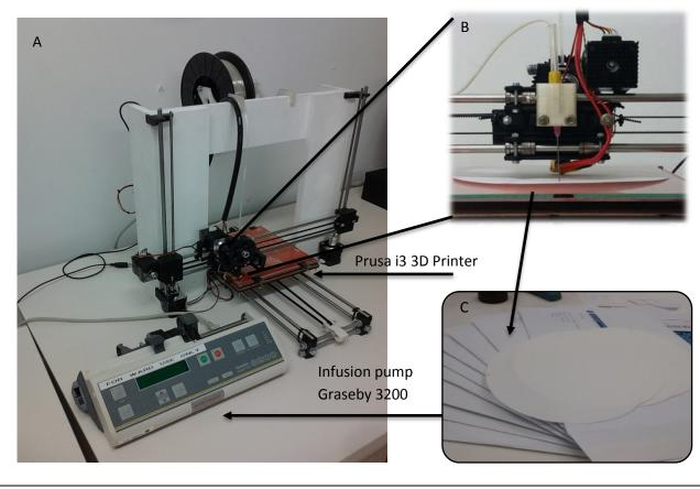
**Figure 1** (a) Schematic of the one-step plotting method for patterning paper with the use of a Prusa i3 printer and a infusion pump Graseby 3200. (b) Detail of the needle adaptor at the Prusa i3. (c) Photo of a manufactured sisal paper.
