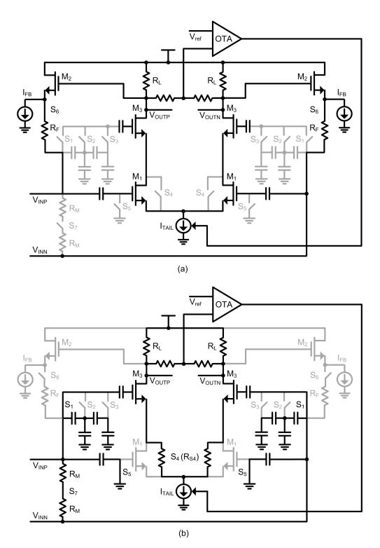
**Figure 5.3:** Schematic of the differential double-input RFPGA with switchable capacitive attenuation (a) Gain setting 1 (b) Gain setting 2
