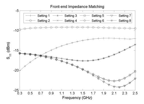
Figure 6.10: Front-end  $s_{11}$  measurement results.
