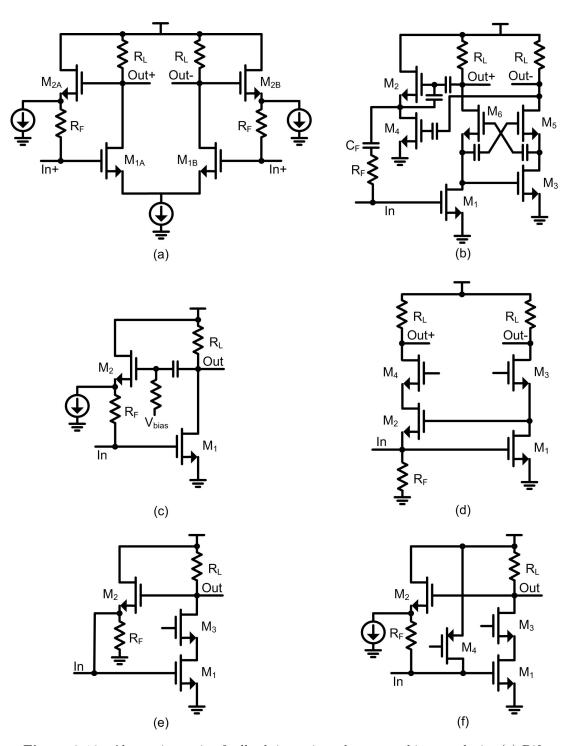
**Figure 3.10:** Alternative active feedback input impedance matching topologies (a) Differential (b) Single-ended to differential conversion with single-branch active feedback (c) AC coupling at the output (d) Single-ended to differential conversion with local feedback (e) Without current source at the feedback (f) Current sink at the input.
