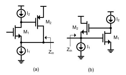
Figure 3.13: Basic topology of an active inductor (a) Using one PMOS and one NMOS transistor (b) Using two NMOS transistors.
