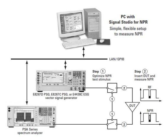
Figure 2.7: Agilent Signal Studio for Noise Power Ratio configuration.
