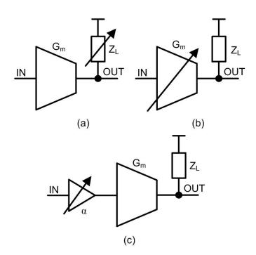
**Figure 3.24:** Configurable-gain amplifier topologies: (a) Variable-load (b) Variable- $G_m$  (c) Pre-attenuation based.
