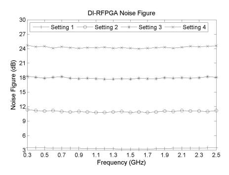
Figure 5.15: DI-RFPGA noise figure measurement results.
