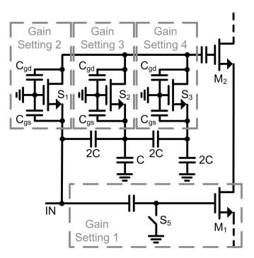
Figure 5.6: Double-input switchable capacitive attenuation using a C-2C ladder and including switch parasitic capacitances.
