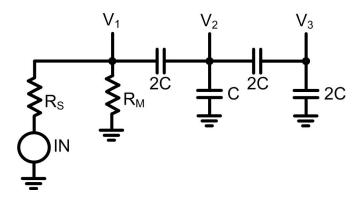
Figure 4.4: Capacitor ladder using a C-2C structure.
