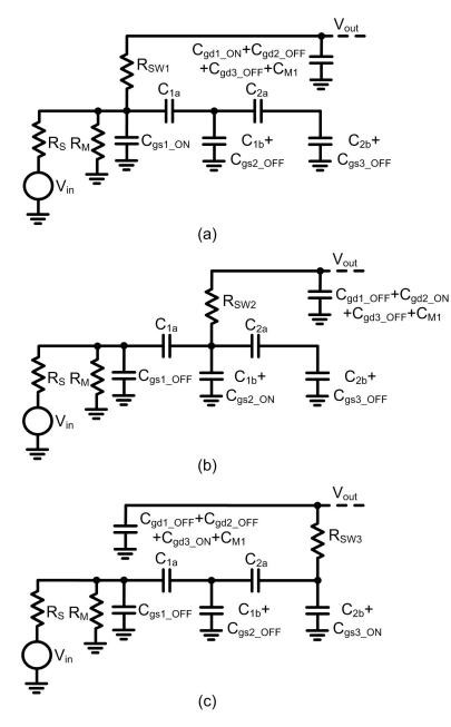
**Figure 4.6:** Circuit model of the capacitor ladder including switch parasitic capacitances and channel resistance for (a) Gain setting 2 (b) Gain setting 3 (c) Gain Setting 4.
