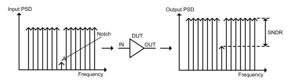
Figure 2.6: NPR measurement process.
