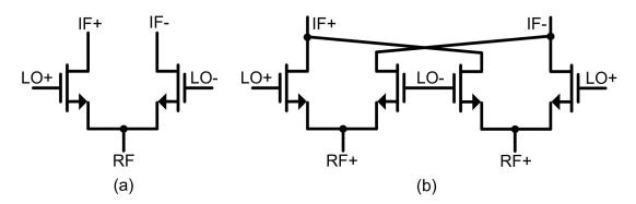
Figure 2.10: Common mixer implementation in CMOS (a) Single-ended (b) Differential.
