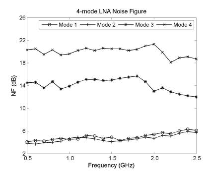
Figure 4.18: Measured noise figure of the RFPGA four settings.
