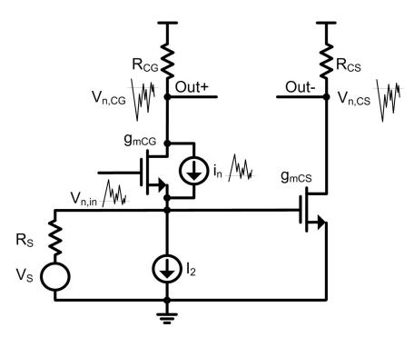
Figure 3.8: Combined common-gate common-source topology providing simultaneous input impedance matching, single-ended to differential conversion and noise-canceling.
