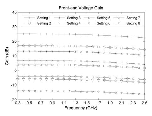
Figure 6.9: Front-end voltage gain measurement results.
