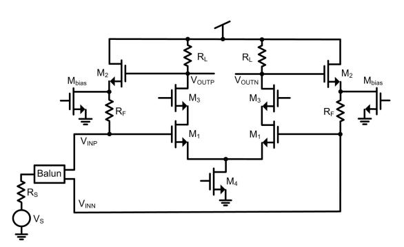
Figure 5.7: DI-RFPGA simplified schematic used for noise calculations at the highestgain setting.
