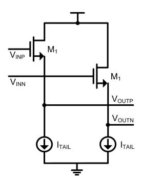
Figure 6.7: Buffers schematic.
