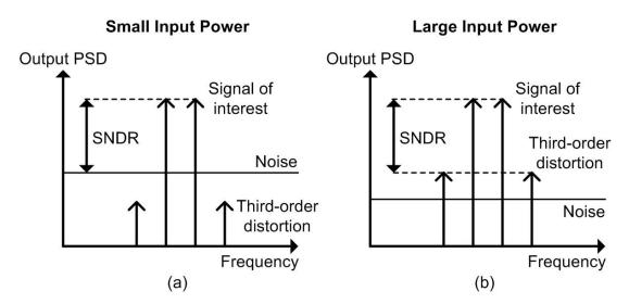
Figure 2.4: SNDR calculation at (a) Small input power (b) Large input power.
