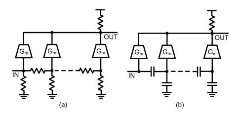
Figure 3.26: Pre-attenuation based amplifier topologies: (a) Resistive (b) Capacitive.
