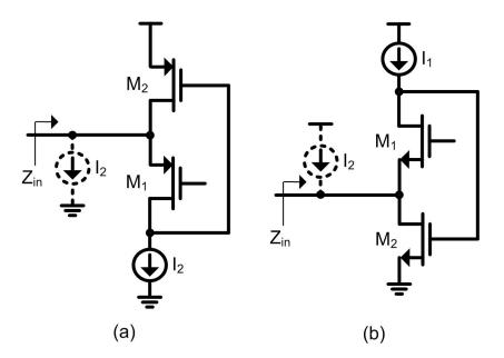
Figure 3.14: Active inductor using the Wu topology (a) PMOS (b) NMOS.
