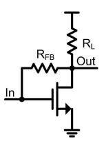
Figure 3.2: Basic topology of the resistive feedback input impedance matching.
