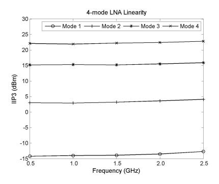
Figure 4.17: Measured IIP3 of the RFPGA four settings.
