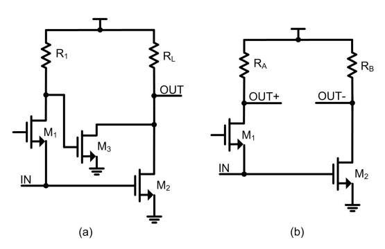
**Figure 3.20:** Noise/distortion cancellation topologies (a) Single-ended (b) Single-ended to differential conversion.
