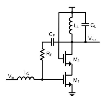
Figure 3.3: Resistive feedback using input inductor.
