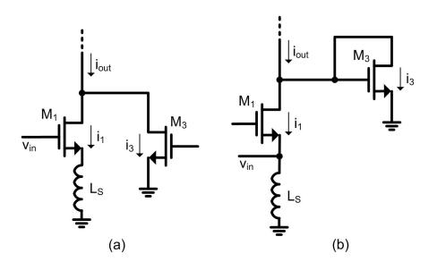
Figure 3.23: Alternative implementation of post-distortion (a) Implementation in [103] (b) Implementation in [102].
