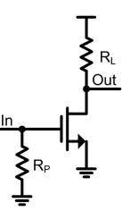
Figure 3.1: Basic topology of the parallel resistance input impedance matching.
