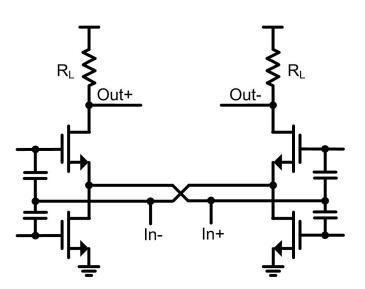
Figure 3.7: Basic topology of the common-gate dual capacitive cross-coupling input impedance matching.
