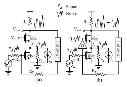
**Figure 3.4:** Resistive feedback using feedforward noise and distortion cancellation [38] (a) Conventional resistive feedback LNA (b) Resistive feedback LNA using feedforward noise and distortion cancellation.
