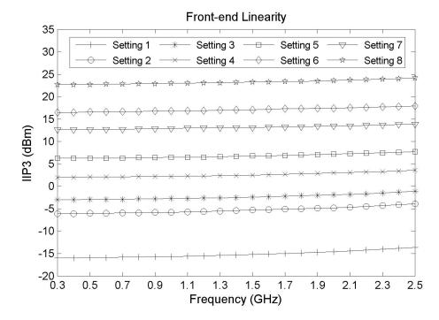
Figure 6.11: Front-end IIP3 measurement results.
