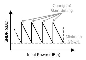
Figure 2.5: SNDR vs input power with constant SNDR steps.
