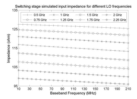
Figure 6.5: Simulated input impedance of the switching stage for different LO frequencies.
