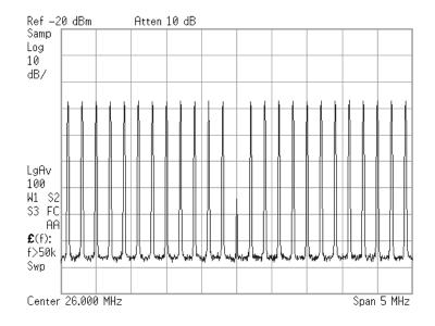
**Figure 6.16:** Instance of the output signal in an NPR measurement (zoom into the carriers). The input signal has a power of 5 dBm and 400 carriers with a 200 kHz spacing centered at 2.05 GHz. The front-end is configured at the lower gain setting with a baseband frequency from 10 MHz to 90 MHz with a notch located at 26 MHz.
