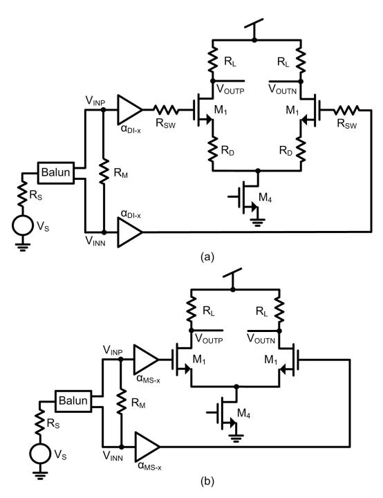
Figure 5.8: Simplified schematics used for noise calculations at attenuation settings (a) DI topology (b) MS topology.
