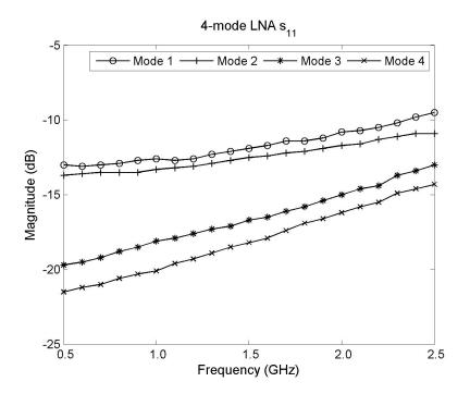
**Figure 4.16:** Measured  $s_{11}$  of the RFPGA four settings.
