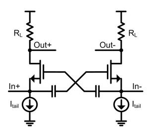
Figure 3.6: Basic topology of the common-gate capacitive cross-coupling input impedance matching.
