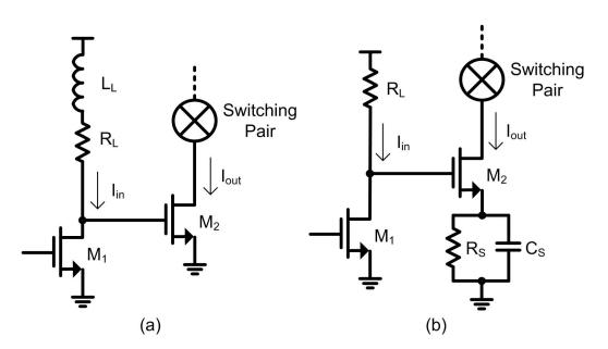
**Figure 3.16:** Techniques for adding a zero in the gain transfer function (a) Inductive peaking (b) Capacitive peaking.
