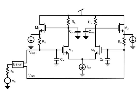
Figure 4.9: LNA1 simplified schematic used for input impedance optimization calculations.
