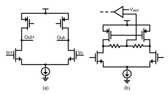
**Figure 3.12:** Basic topologies of a circuit with active loads (a) Differential amplifier with PMOS loads (b) Differential amplifier with active loads and CMFB.
