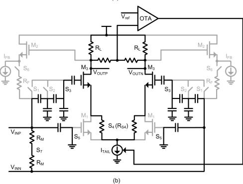
**Figure 5.4:** Schematic of the differential double-input RFPGA with switchable capacitive attenuation (a) Gain setting 3 (b) Gain setting 4
