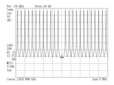
**Figure 6.15:** Instance of the input signal in an NPR measurement (zoom into the carriers). The input signal has a power of 5 dBm and 400 carriers with a 200 kHz spacing centered at 2.05 GHz with a notch located at 2.026 GHz.
