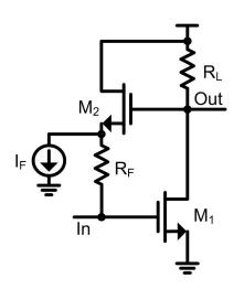
Figure 3.9: Basic topology of the active feedback input impedance matching.
