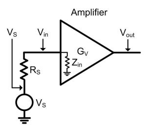
Figure 4.10: Input structure of a front-end.
