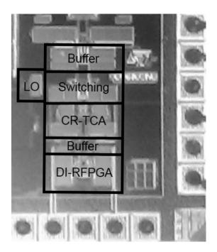
Figure 6.8: Front-end prototype microphotograph.
