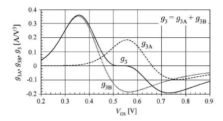
Figure 3.18: Derivative superposition technique [91]: Third-order coefficients of the main and auxiliary transistors in the derivative superposition method.
