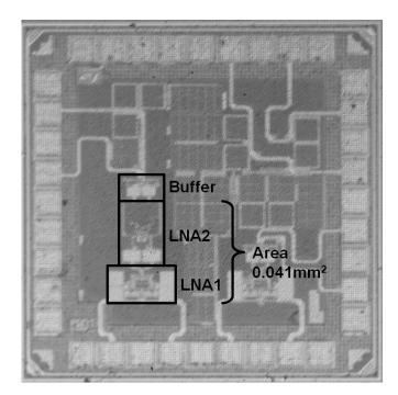
Figure 4.14: Microphotograph of the RFPGA.
