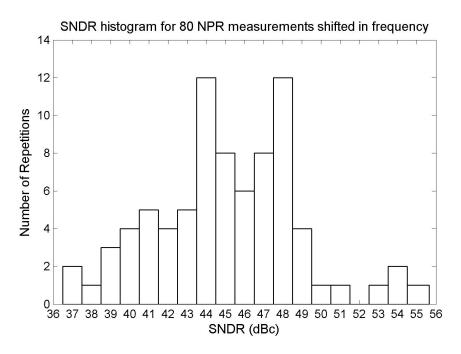
Figure 6.19: Histogram of the NPR notch measurements.
