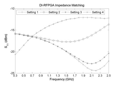
Figure 5.13: DI-RFPGA  $s_{11}$  measurement results.
