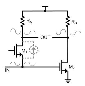
Figure 3.21: Signal phases in the noise/distortion cancellation topology: fundamental signal in solid line and noise/distortion in dashed line.
