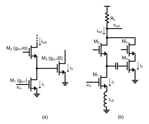
**Figure 3.22:** Basic topology of the post-distortion technique (a) Core components (b) Implementation in [101].
