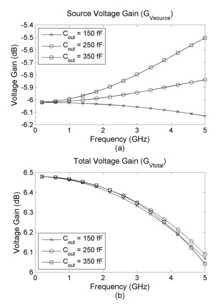
Figure 4.12: Voltage gain using the active feedback input impedance matching topology for different values of output capacitance (a) Source voltage gain (b) Total voltage gain (source plus amplifier).
