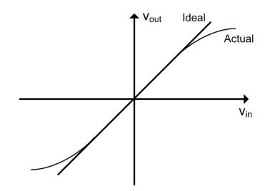
Figure 2.1: Actual versus ideal behavior of an amplifying device.
