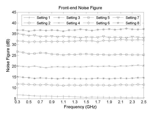
Figure 6.12: Front-end noise figure measurement results.
