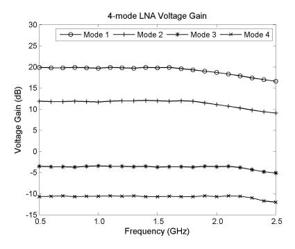
Figure 4.15: Measured voltage gain of the RFPGA four settings.
