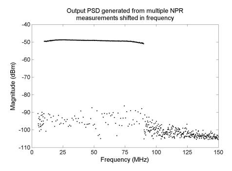
Figure 6.18: Full channel output spectrum containing all the individual NPR notch measurements.
