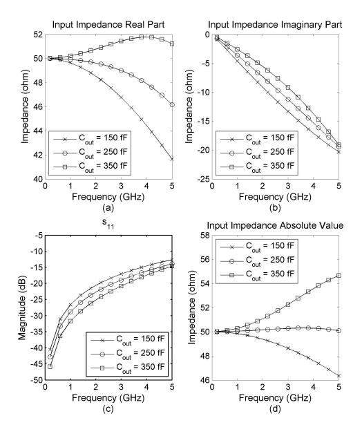
**Figure 4.11:** High frequency behavior of the active feedback input impedance matching topology for different values of  $C_{out}$ : (a) Real part of the input impedance (b) Imaginary part of the input impedance (c)  $|s_{11}|$  in dB (d) Absolute value of the input impedance.
