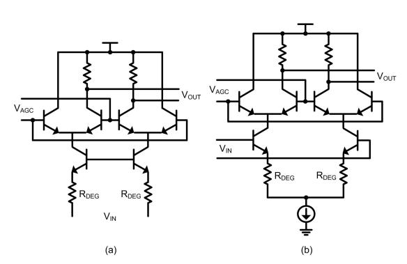
**Figure 3.25:** Variable- $G_m$  amplifiers with current steering and degeneration: (a) Common-gate (b) Common-source.
