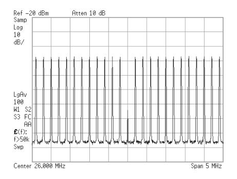
Figure 2.9: Sample screenshot of a front-end output NPR measurement zooming into the notch.
