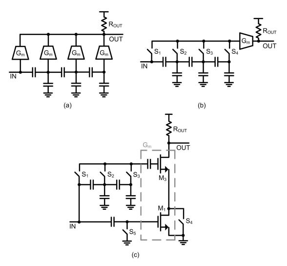
Figure 5.1: Implementations of capacitive attenuation PGAs: (a) Non-switchable (b) Switchable (c) Double-input switchable.
