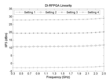
Figure 5.14: DI-RFPGA IIP3 measurement results.
