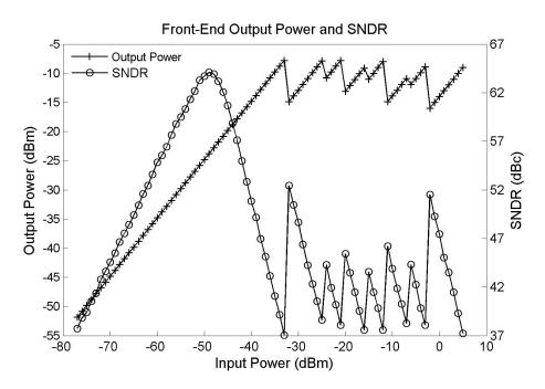
Figure 6.17: SNDR and output power evolution versus input power.
