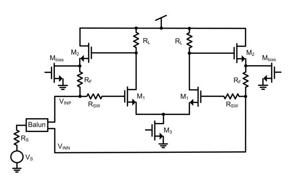
Figure 4.7: LNA1 simplified schematic used for noise optimization calculations.
