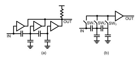
Figure 4.1: Capacitive attenuation topology, (a) Nonswitchable (b) Switchable
