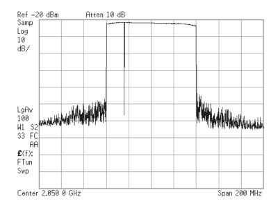
Figure 6.13: Instance of the input signal in an NPR measurement (full channel view). The input signal has a power of 5 dBm and 400 carriers with a 200 kHz spacing centered at 2.05 GHz.
