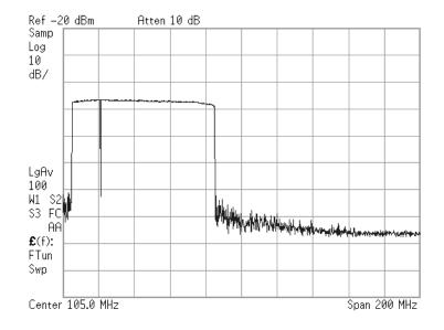
**Figure 6.14:** Instance of the output signal in an NPR measurement (full channel view). The input signal has a power of 5 dBm and 400 carriers with a 200 kHz spacing centered at 2.05 GHz. The front-end is configured at the lower gain setting with a baseband frequency from 10 MHz to 90 MHz.
