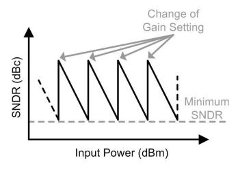
Figure 6.6: SNDR vs input power with constant SNDR steps.
