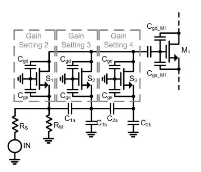
Figure 4.5: Capacitor ladder including the parasitic capacitances of the switches.
