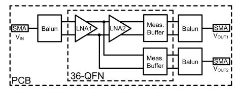
Figure 4.13: PCB measurement setup.
