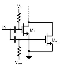
Figure 3.17: Derivative superposition structure.
