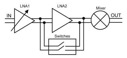
Figure 4.3: Proposed configuration of RFPGA prototype I in a front-end implementation.
