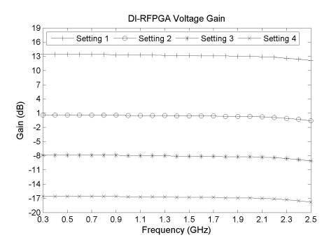
Figure 5.12: DI-RFPGA voltage gain measurement results.
