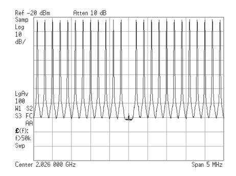
Figure 2.8: Sample screenshot of NPR input signal after applying pre-distortion zooming into the notch.
