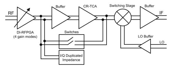
Figure 6.3: Architecture of the implemented front-end.
