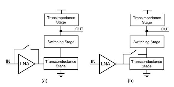
**Figure 6.2:** (a) Front-end with by-passable LNA and (b) Front-end with by-passable mixer transconductance.
