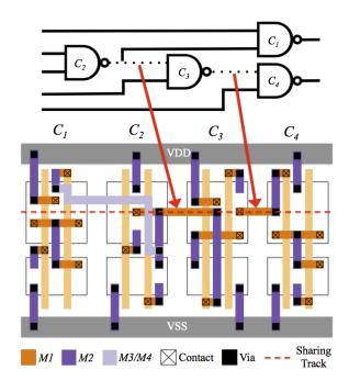
Figure 2: Small circuit consisting of four NAND gates
