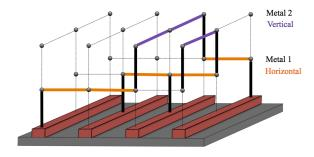
Figure 3: Grid representation for internal cell routing
