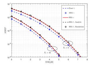
Fig. 3. Average bit error probability of the proposed system at  $N_t = 32$ ,  $N_a = 4$ , 16-PSK, perfect and estimated thresholds.
