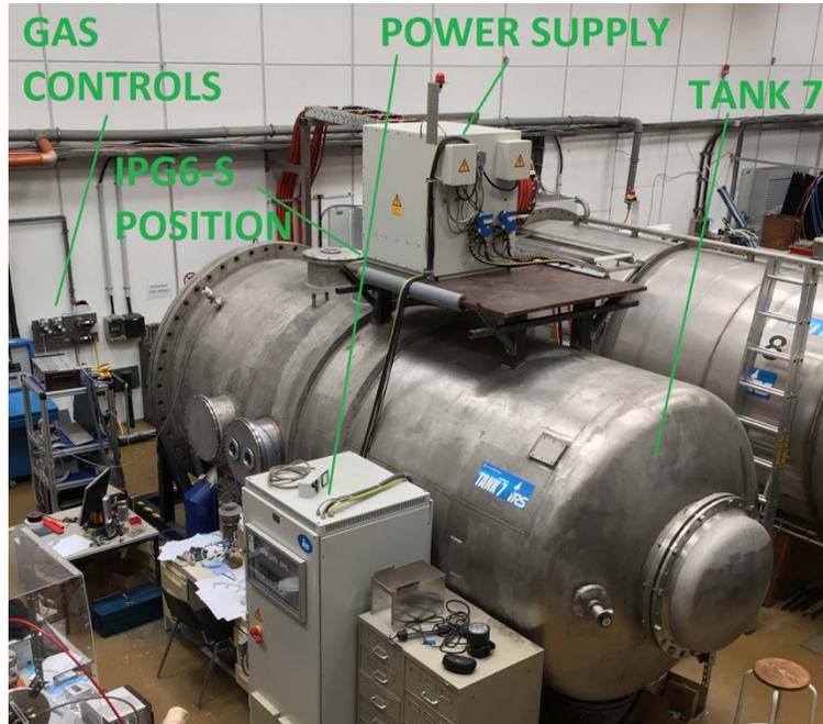
Fig. 4 IPG6-S refurbished facility
