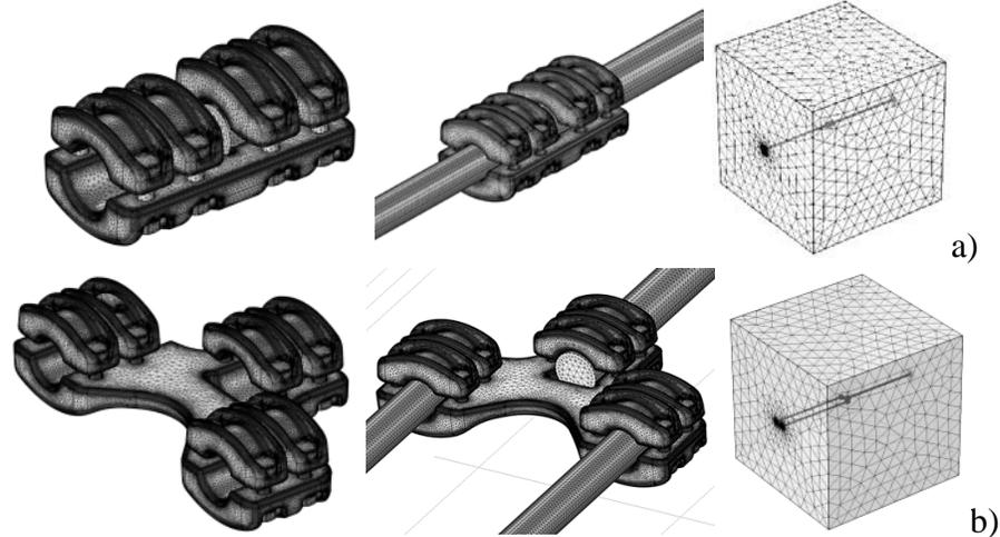
Fig. 2. Substation connectors analyzed. Geometry and meshes applied in the FEM simulations. a) Connector J40S33PK. b) Connector J40S33D4PK.
