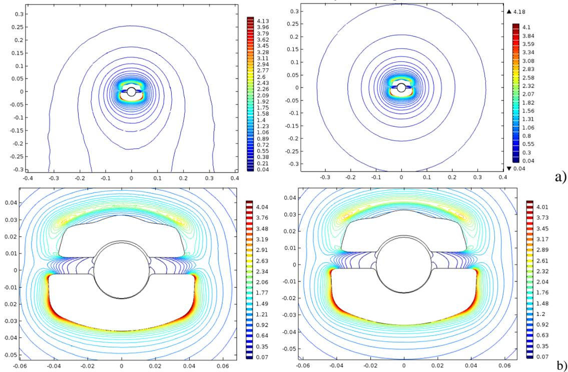
Fig. 7. a) Electric field (kV<sub>peak</sub>/mm) distribution around the most stressed parts of the connector for the connector placed at a height of 0.315 m and 7 m above the ground plane, respectively. b) Detail of the electric field distribution on the vicinities of the surface of the connector for both configurations, 0.315 m and 7 m above the ground plane, respectively.
