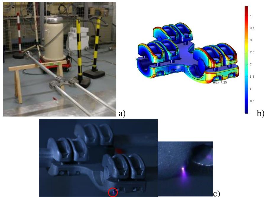
Fig. 9. Connector J40S33D4PK. Small-size unscreened laboratory. a) Experimental setup of the simplified visual corona test including the tested substation connector, the conductors and the spherical corona protections. The height above ground plane is 0.455 m. b) FEM simulation of the J40S33D4PK mechanical substation connector. The electric field strength is given in  $kV_{peak}/mm$ . c) Visual corona photographed with the digital camera.
