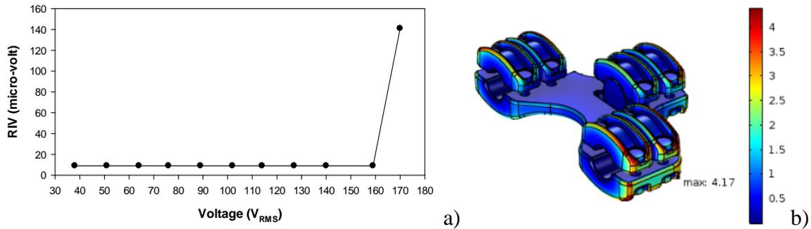
Fig. 8. Connector J40S33D4PK. Large-size screened laboratory. The height above ground plane is 7 m. a) RIV measurement to determine the corona inception voltage conducted in Veiki Laboratory. b) FEM simulation. The electric field strength is given in  $kV_{peak}/mm$ .
