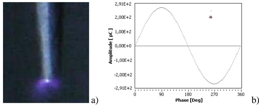
Fig. 4. Detection limit of the needle-plane setup. a) Alternating current negative corona photograph taken with the digital camera. b) Partial discharge pattern corresponding to negative corona acquired during 39.55 s (310 pulses) with the PD detector.
