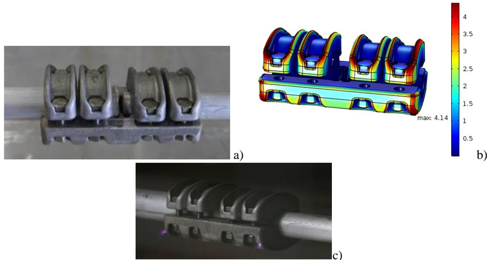
Fig. 6. Connector J40S33PK. Small-size unscreened laboratory. The height above ground plane is 0.315 m. a) Experimental setup of the simplified visual corona test including the tested substation connector, the conductors and the spherical corona protections. b) FEM simulation of the J40S33PK mechanical substation connector. The electric field strength is given in  $kV_{peak}/mm$ . c) Visual corona photographed with the digital camera.
