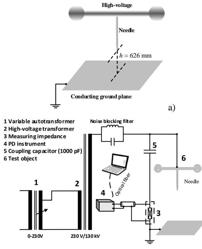
Fig. 3. a) Needle-plane experimental setup to calibrate the digital camera against PD measurements. The rod of the needle has a diameter of 3 mm, whereas the diameter of the tip is 1.5 mm. The distance between the tip of the needle and the ground plane is 626 mm. b) PD measuring circuit in accordance with the IEC60270 standard.
