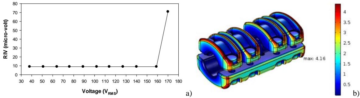
Fig. 5. Connector J40S33PK. Large-size screened laboratory. The height above ground plane is 7 m. a) RIV measurement to determine the corona inception voltage conducted in Veiki Laboratory. b) FEM simulation. The electric field strength is given in  $kV_{peak}/mm$ .
