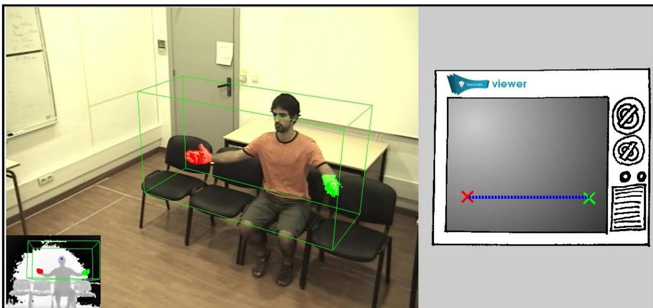
Hand tracking using the Time-Of-Flight camera with visual feedback to the user
