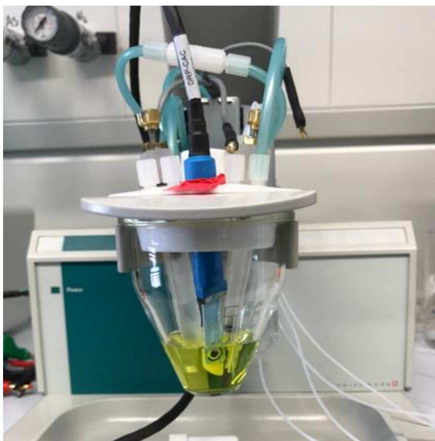
Figure 9. Deposition of \text{UO}_2 on dropsen electrode surface
