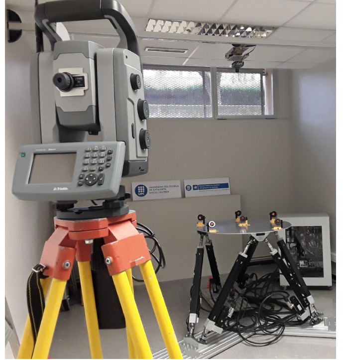
Fig. 5. Calibration process by using an electronic theodolite
