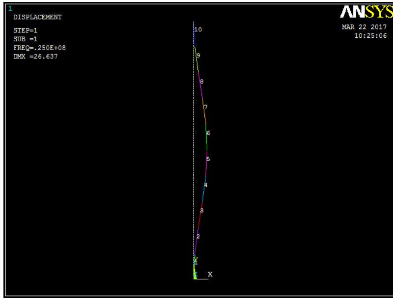
Figure 46: First mode of buckling. Composite column.
