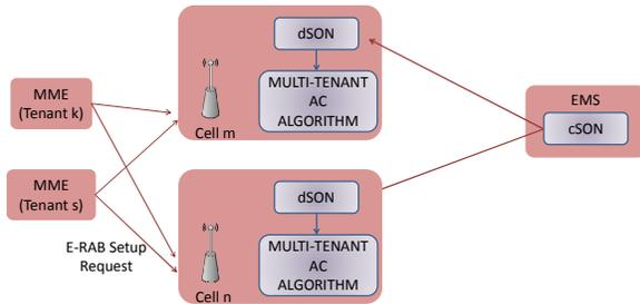
Fig. 1. Functional architecture of the AC Self-Optimization
