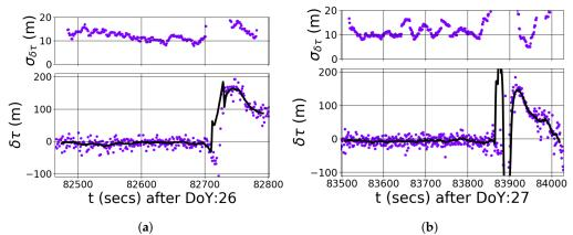
**Figure 6.** The differential delays  $\delta \tau$  and their standard deviation  $\sigma_{\delta \tau}$  obtained from the whole data set, after correcting for the trend derived from the sea waveforms. Superimposed to the values  $\delta \tau^{\text{sea}}$  we include a running mean used to derive  $\sigma_{\delta \tau}$ . (a) 26 January 2015. (b) 27 January 2015.
