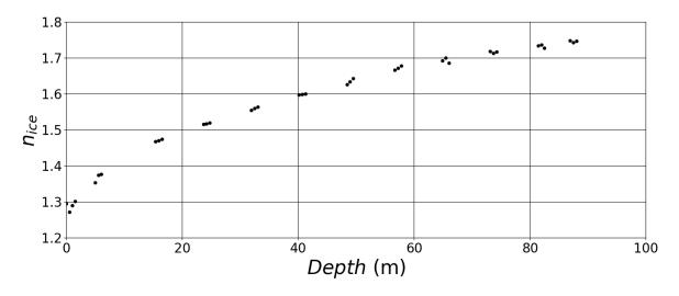
**Figure 8.** Refractive index as a function of ice depth, as reported in Table 4 of Ref [45], estimated from North Greenland Eemian Ice Drilling (NEEM) camp data.
