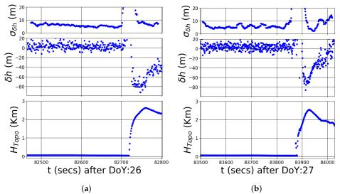
**Figure 7.** In each column we have represented from bottom to top (1) the topography associated to each track  $H_{Topo}$ , (2) the estimate of the *apparent* the height relative to the *a priori* model  $\delta h^{\text{apparent}}$ , and (3) its standard deviation  $\sigma_{\delta h}$ . (a) 26 January 2015. (b) 27 January 2015.
