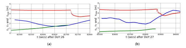
**Figure 3.** The modeled delays due to tidal  $\tau_{tides}$  (green), ionospheric  $\tau_{I}$  (blue) and tropospheric effects  $\tau_{T}$  (red), are represented for the two transects. (**a**) 26 January 2015. (**b**) 27 January 2015.
