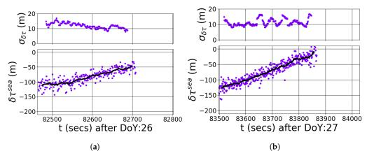
**Figure 5.** The observed delays  $\delta \tau^{\text{sea}}$  and their standard deviation  $\sigma_{\delta\tau}$  obtained from the sea waveforms. Superimposed on the values  $\delta \tau^{\text{sea}}$  we include a running mean used to derive  $\sigma_{\delta\tau}$ . The trend in the observed delays is attributed in this study to effects of TDS-1 clock inaccuracies. (a) 26 January 2015. (b) 27 January 2015.
