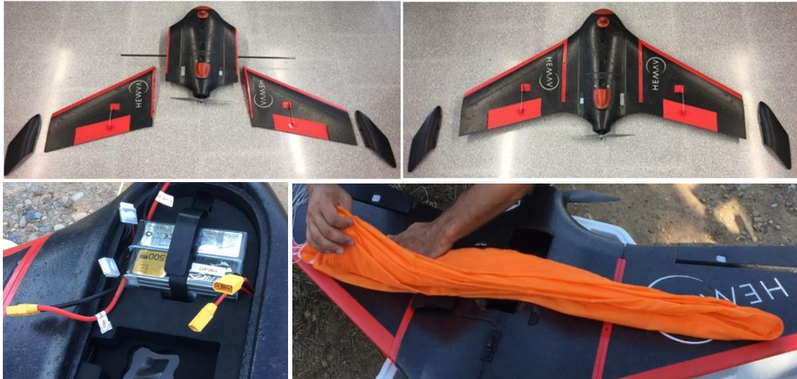
Fig. 3.11. Preparation of the HP2 airframe
