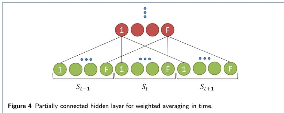
Figure 4 Partially connected hidden layer for weighted averaging in time.
