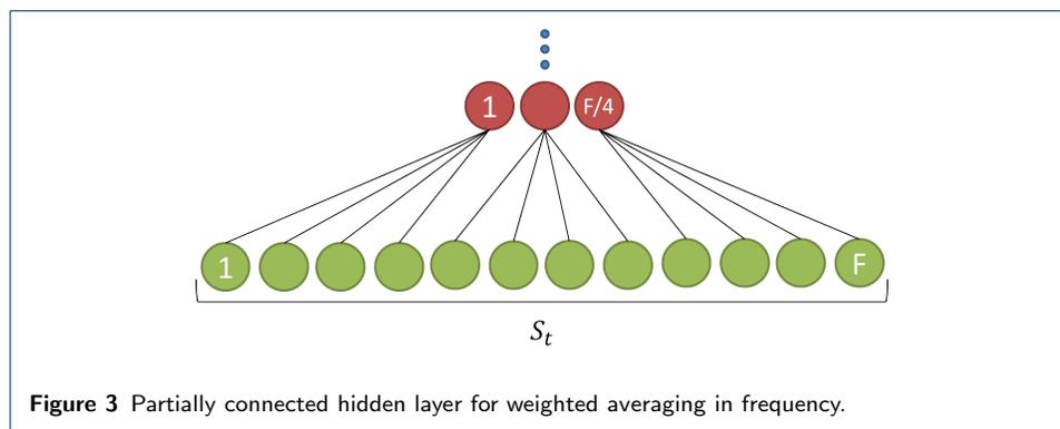
Figure 3 Partially connected hidden layer for weighted averaging in frequency.
