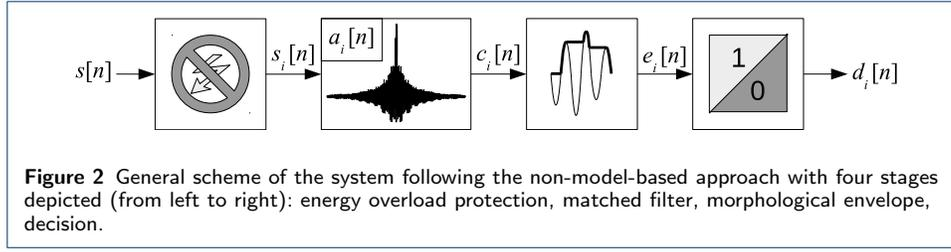
**Figure 2** General scheme of the system following the non-model-based approach with four stages depicted (from left to right): energy overload protection, matched filter, morphological envelope, decision.
