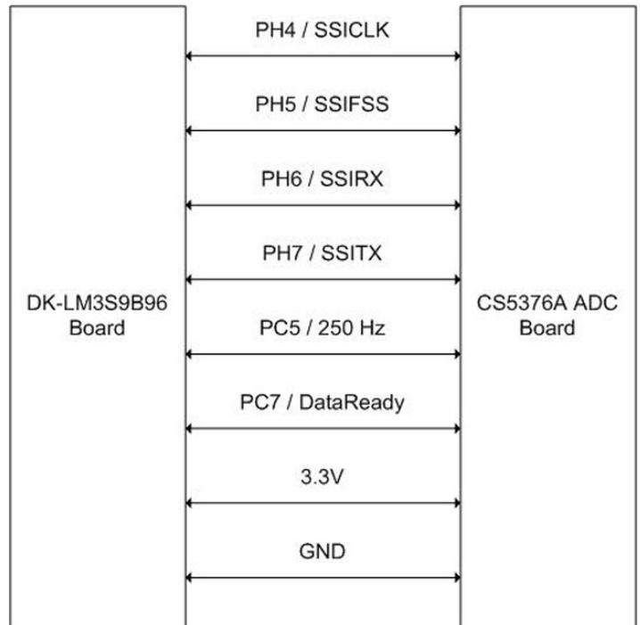
**Figure 2: Connection between DK-LM3S9B96 and CS5376A**
