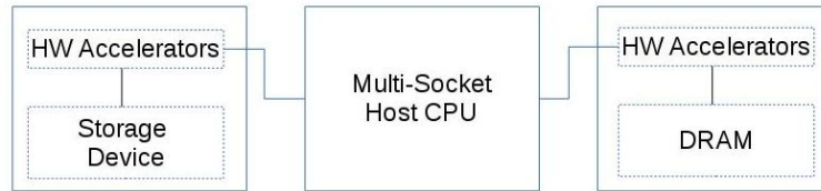
Figure 9.1: NDC Supported Single Node in Scale-in Clusters for in-Memory Data Analytics with Spark
