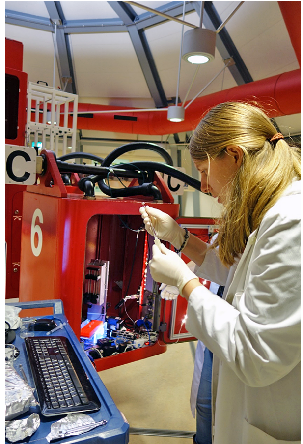
Preparing a syringe for hypergravity droplet generation (Photo credit: ESA).
