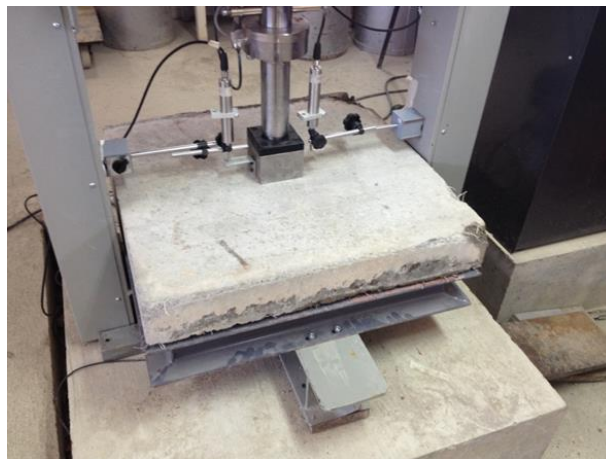
Figure 1. View of EFNARC panel test.
