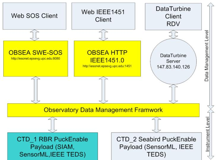
(before) **Figure 2 Access to real-time data using standards like SWE SOS or IEEE1451**
