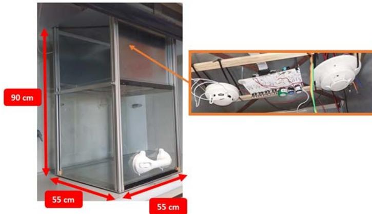
Fig. 1. The developed multi-sensor platform was placed on 272-liter measurement chamber in which different type of fires and nuisances were performed. Two commercially available fire alarms based on smoke detection were also integrated in the measurement chamber.
