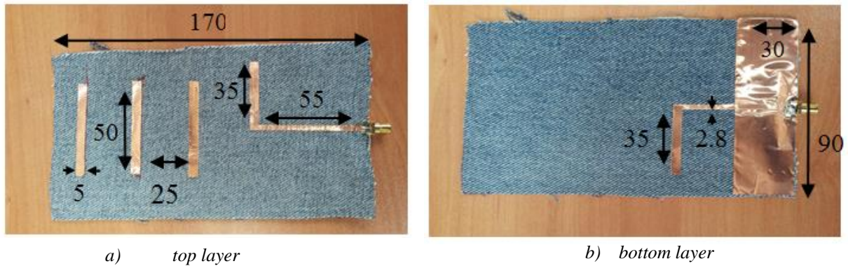
Figure.1 Geometry (dimensions in mm) of the proposed Textil Yagi.Antenna.
