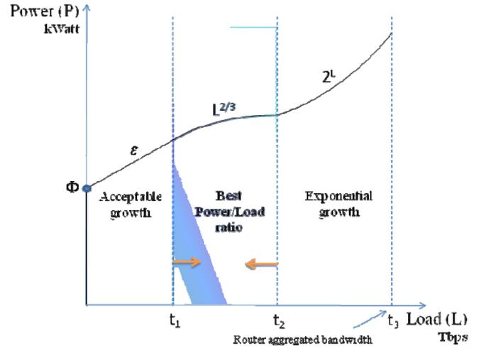
Figure 3. Power consumption in combined power consumption model.
