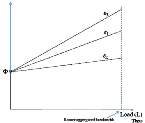
Figure 1. Power consumption in linear power consumption model.
