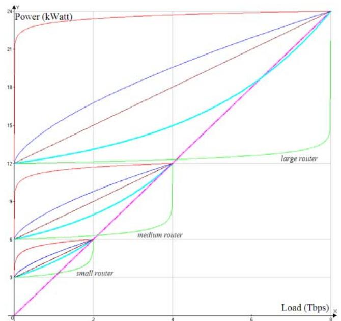
Figure 5. Power consumption functions for various size electronic routers.
