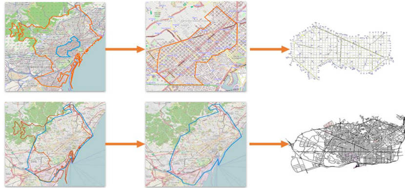
Figure 6. Top: Example area (left), simulation test-site (center), and the Aimsun model (right). Bottom: Inner ring area of Metropolitan Barcelona (left), simulation test-site (center), Aimsun model (right).
