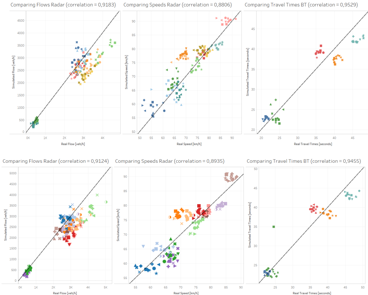
Fig. 2. Top: Simulated vs. Real in Calibration dataset (a) Flows; (b) Speeds; (c) Travel Times. Below: Simulated vs. Real in Validation dataset (a) Flows; (b) Speeds; (c) Travel Times
