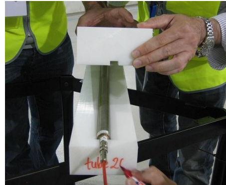
Figure 2. View of one of the PE blocks with ^3\text{He} tube used in the neutron background measurement at LSC.
