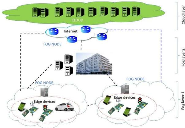
Figure 2. Fog to Cloud (F2C) computing architecture
