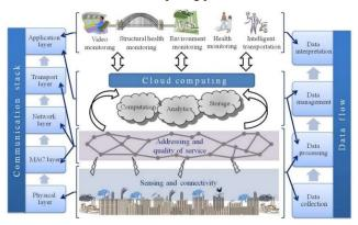
Figure 1. IoT architecture for Smart City [6].
