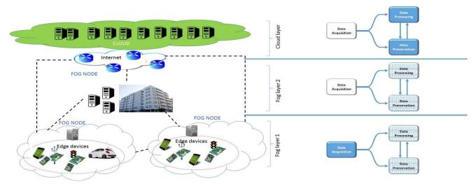
Figure 6. Illustration of the SCC-DLC model, a COSA-DLC adaptated to a Smart City.
