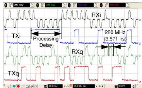
Figure 8. Datagram measurements of the transmitted bits and the demodulated signals at 560 Mbps.
