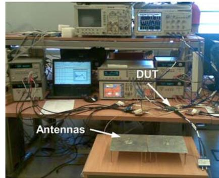
Figure 7. Measurements testbench setup.
