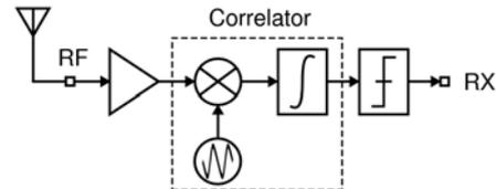
Figure 2. Architecture for the IR-UWB correlator-based receiver.
