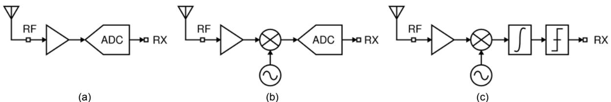
Figure 1. Receiver architecture for (a) software radio (b) software radio with reduced requirements and (c) superheterodyne architecture.
