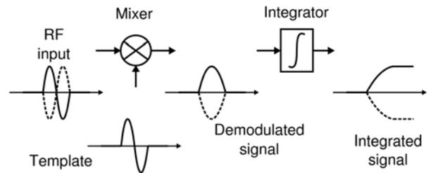
Figure 3. Impulse radio correlator operation.
