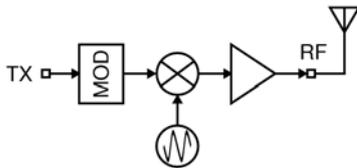
Figure 4. Architecture for the UWB impulse radio transmitter.
