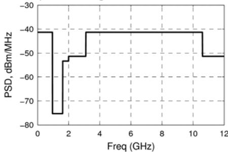
Figure 1. UWB Spectral Mask FCC part 15 regulations.
