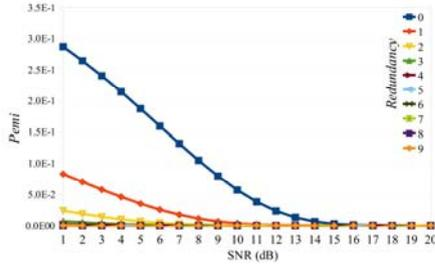
Figure 3. Error probability for a single gate with 0-9 port redundancies.
