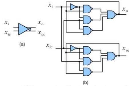
Figure 4. NOT gate using TL with redundancy of one as well as complementary data. (a) Symbol, and (b) Schematic view.
