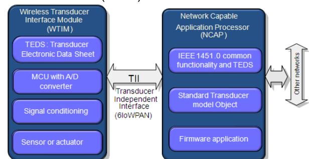
Figure 2. IEEE 1451 Smart sensor model
