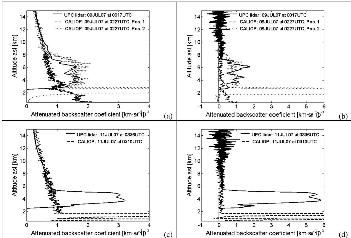
Fig. 11. Total attenuated backscatter coefficient on 09JUL07 at (a) 532 and (b) 1064 nm, and on 11JUL07 at (c) 532 and (d) 1064 nm. The lidar-derived *AOT* on 09JUL07 is 0.145 and 0.046 at 532 and 1064 nm, respectively. On 11JUL07 it is, respectively, 0.313 and 0.19.
