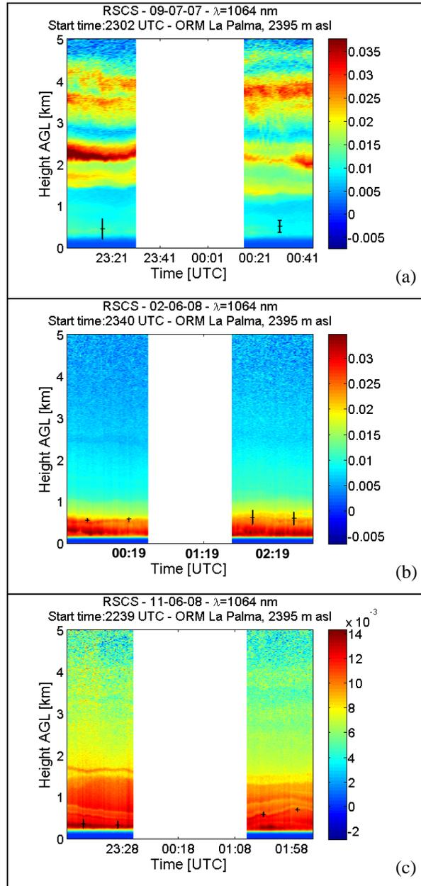
Fig. 3. Temporal evolution of the RSCS on (a) 09JUL07, (b) 02JUN08 and (c) 11JUN08. The PBL height is indicated by '+' signs. The error bar associated to the PBL height was computed as the standard deviation of the 30 profiles used to calculate the mean PBL height.
