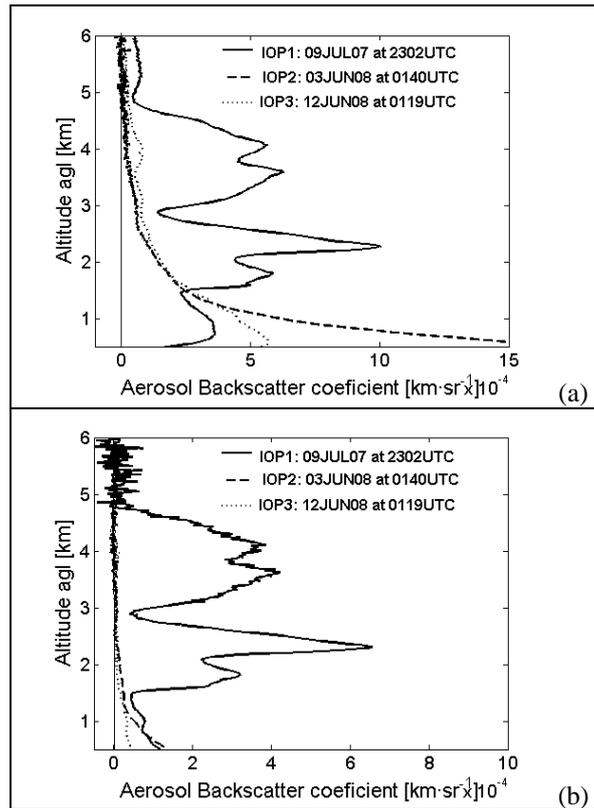
Fig. 8. Aerosol backscatter coefficient at (a) 532 nm and (b) 1064 nm. The *AOT* at 532 nm for 09JUL07, 03JUN08 and 12JUN08 is 0.118, 0.055 and 0.032, respectively. At 1064 nm it is 0.06, 0.0039 and 0.0022, respectively.
