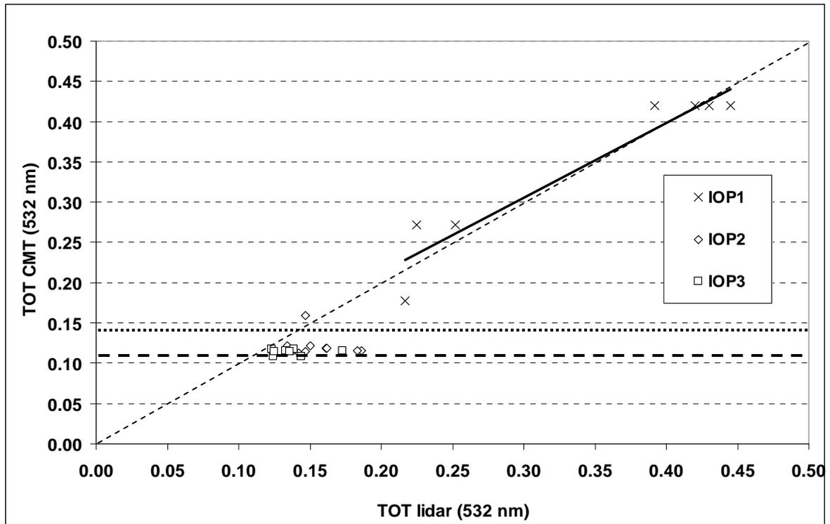
Fig. 9. CMT-derived vs. lidar-derived *TOT* at 532 nm. The dashed and dotted horizontal lines indicate the CMT-derived *TOT* (532 nm) limits for no atmospheric extinction at all (0.1105, conversion in *TOT* of 0.12 mag·aimass<sup>-1</sup>) and Saharan dust presence (0.1409, conversion in *TOT* of 0.153 mag·aimass<sup>-1</sup>), respectively. The solid black line corresponds to the best fit between lidar- and CMT-derived *TOT* for IOP1.
