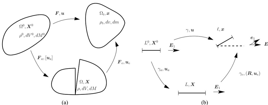
Figure 1: Maps between the reference configuration, the relaxed configuration, and the deformed configuration for the continuum model (a), and the truss model (b).
