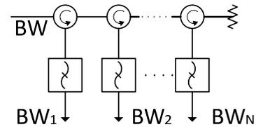
Fig. 6. Multiplexing architecture based on a Circulator-Coupled approach.
