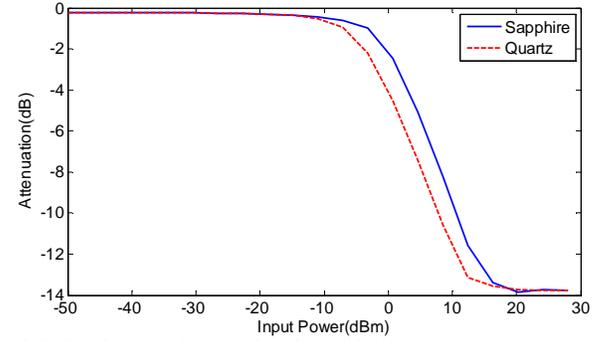
Fig. 9. In-band attenuation as a function of the input power
